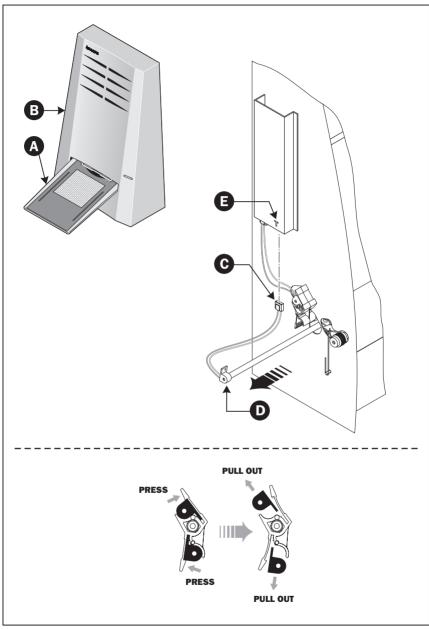
Figure 9: Replacing the Light Tubes
